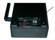
As seen through opening, right 2 switches set machine signal
